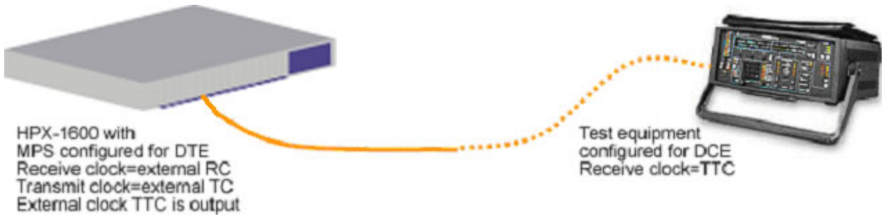
Figure 2 : DTE testing using FireBERD in DCE mode
